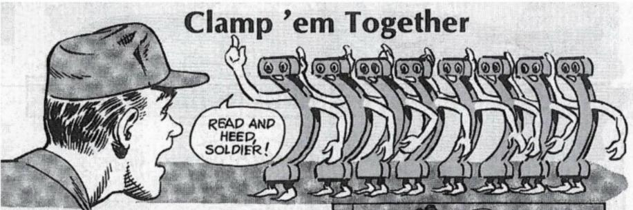
When you remove the tail rotor drive shafts on your Huey or Cobra, you want to keep the 2 numbered coupling clamp halves together because they're a matched set.
