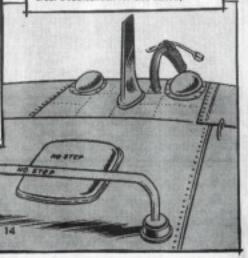
CABIN TOP-Holes, rips, tears, buckling. Ventilators get a second look. Anyone put his brogans thru 'em? Same goes for NO-STEP spots, Ventsclogged. Broken, damaged antennas and anti-collision
