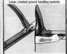
LANDING GEAR-Damaged steps and fittings. Deep scratches, scuffs, nicks, dents
