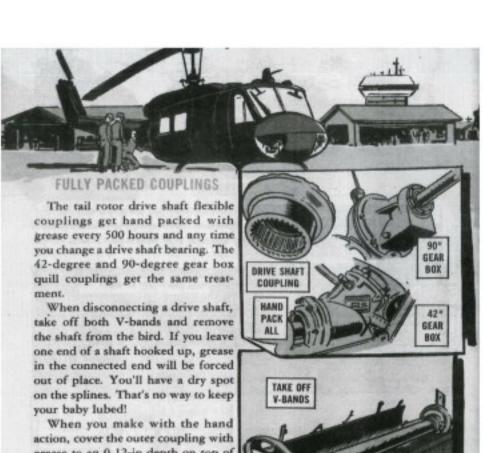
grease to an 0.12-in depth on top of the internal splines over the exposed full length.
