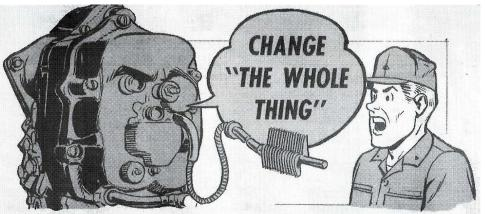
A complete T53 engine fuel control unit includes the  $T_1$  temperature sensing element.
