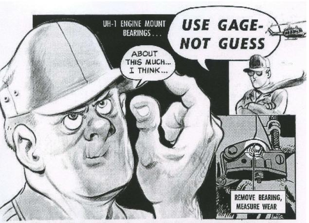
That's right, chopper caretakers. TM 55-1520-210-20PMP (26 Apr 68) says engine mount bearings get replaced if allowable play limits—0.006-in radial, 0.012-in axial—are exceeded.
