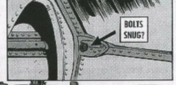
After you c-a-r-c-f-u-l-l-y check around the bolt holes for hairline cracks, distortion, corrosion, and damage, take a good look at each bolt.
