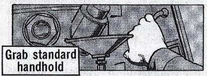
Latch onto the engine cowling hinge with your left hand.
