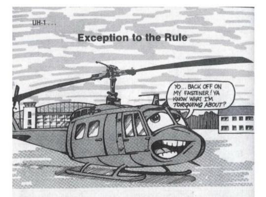
The general rule on torquing and retorquing is to back off the fastener before tightening with a torque wrench.
