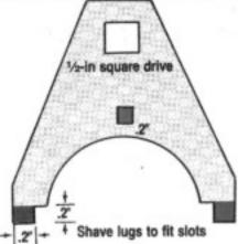
It should be identical to spanner wrench, NSN 5120-00-421-7401, that's Item T60 in Table 1-2 of the TM, except for the size of the lugs. The lugs should be shaved to fit snugly into the grip nut's slots.
