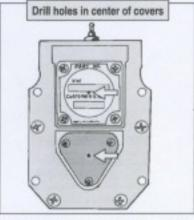
4. Drill a third hole in the top center of the converter body using drill bit size R .339.
