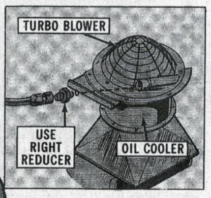
A reducer that provides an increased air flow is used on the production AH-1S Model and AH-1G's modified to the "S" Model. Never use the increased flow reducer on other Cobra's and Huey's because the fan will overspeed and may tear apart.
