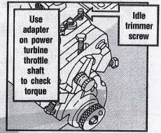
Torque limits are up to 15 lb-in for the 0° to 100° travel and 25 lb-in from 100° to 0° travel (cutoff). Limits of adjustment are reached when cutoff cannot be obtained.
