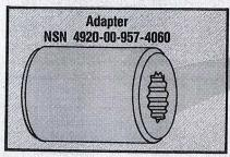
The adapter is used with a standard torque wrench on the power turbine throttle shaft to check torque following each 1/8 counterclockwise adjustment of the idle trimmer screw.
