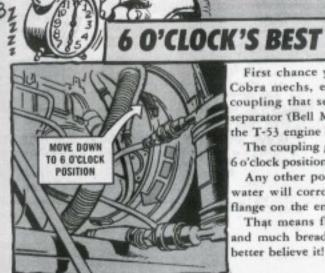
First chance you get, Huey and Cobra mechs, eyeball the V-band coupling that secures the particle separator (Bell Mouth Assembly) to the T-53 engine housing.
