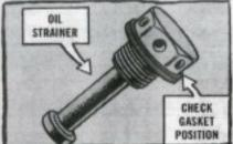
Forget about adding an O-ring. Take a look at the strainer gasket. If it's in wrong, with the recessed side down, get a new gasket. Put it in the right way, recessed side up. That'll stop the leak.
