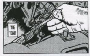
Easiest way to avoid dangle anguish is to re-tie any cable or wiring spot ties you remove, break, or otherwise disturb.
