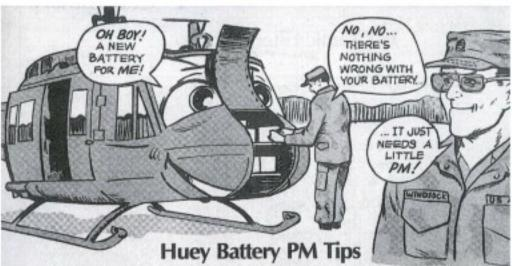
When you check a battery and find the recessed pins in the receptacle. water or electrolyte on the cells, don't get in a hurry to exchange the battery. The wet stuff could just be condensation or spilled electrolyte. So, before you exchange the power package for a new \$885 battery, pull your PM like it says in Para 4-6 of TM 11-6140-203-14-2.
