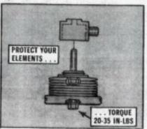
So, follow Para 5-99 of TM 55-2840-229-24 (Apr 71), the engine manual. The attaching bolt gets a special torque of 20-35 inch-pounds-no more.
