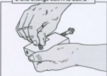
2: Disengage tool, remove bolt C and change bolt A to bolt B
