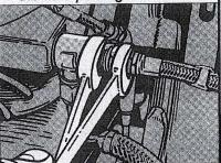
—Disconnect the nut on the 3&4 oil bearing line (Item 11, Fig 64, TM 55-2840-229-23P) with a 9/16-in wrench.
