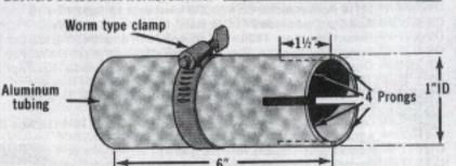
ing. Just latch onto a hack saw and cut down on the tool prongs. 2 slots (4 prongs) to the depth indicated. Add a suitable worm type as you please! clamp over the tube.
