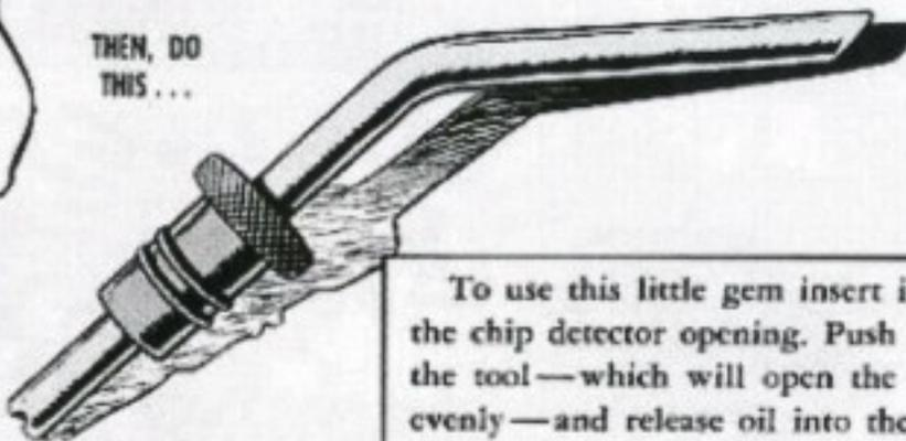
Slip the packing ring and a salvaged chip detector plug over the tube and your tool is complete.
