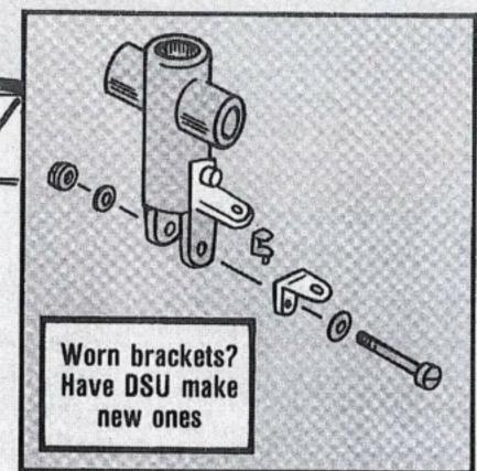
replacement bracket. However, your sheetmetal shop can make it by following the details in Figs D-215 and D-216 of TM 55-1520-210-23.
