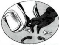
expanding external rings and overcompressing internal rings. Taking time to adjust the stop is quicker than running back to the parts room for a new ring to replace the one you ruined.
