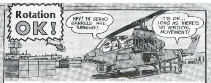
When you Cobra hotshots make with a "hands on" check of the main rotor dual hydraulic servo cylinders during inspections, it's no sweat if the cylinder barrels turn. If there is no vertical movement, the servos are serviceable.
