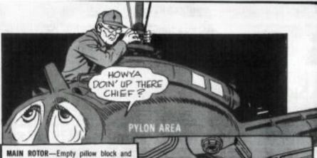
grip oil reservoirs. These pillow block reservoirs can be put on upside down. Watch for this Murphy and for oil leakage and contamination. Nicks, gouges, cuts on hub assembly, blade grips, pitch horns, drag braces.
