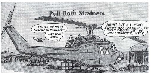
Huey mechs have been faithfully pulling the fuel control servo strainer and replacing the filter on the Phase inspection. The strainer is also cleaned at other flight times, as spelled out in Para 12-22 of TM 55-2840-229-24 (Apr 71) on your Huey T53-L13 engine.
