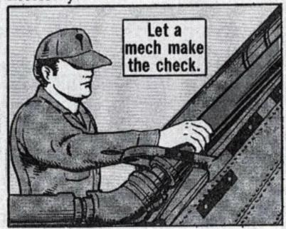
Their idea of using upward pressure on the shaft is to see if the helical spring and spacer used in the 90degree gear box quill is "present 'n' accounted for."
