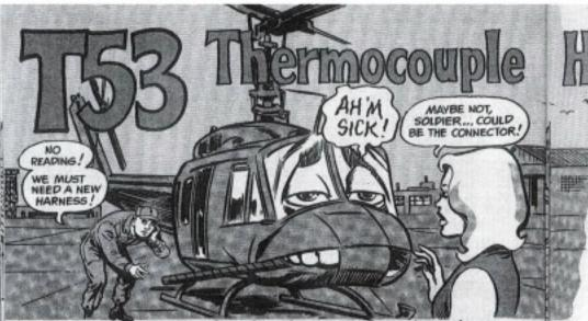
When you don't get readings from the temperature-sensing probes on your Huey or Cobra engine, never rush to change the thermocouple harness. It may be OK.
