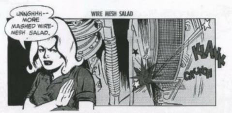
That 2-piece squirrel cage air-inlet screen covering your Huey engine intake bellmouth is designed to keep a snootful of gunk out of the turbine. Does a good job, too, as long as it stays put and doesn't drop down onto that whirling short shaft.
