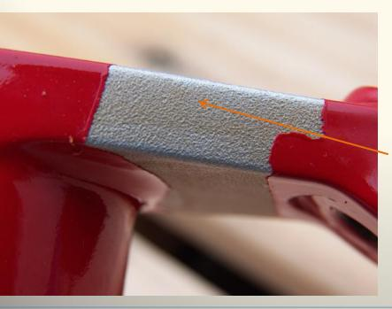
Unworked, peened, alodined surface with no corrosion
