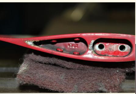
Service Bulletin says "Any corrosion" in the specified area is cause for rejection.
