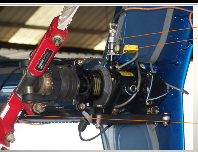
Accelerometer holding photocell in bracket in breather plug tapped hole.
