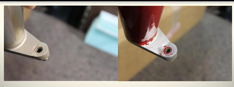
Good spot face showing no scratches No corrosion when stripped
