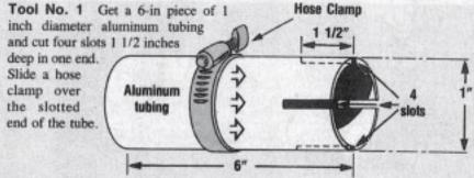
To use the tool, remove the lock ring from the sight glass. Slip the tool over the glass and tighten the clamp. A slight pull removes the glass from the gage.
