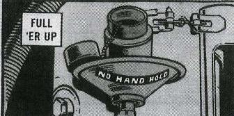
To check leakage, fill up the engine oil tank before a mission of 1 or 2 hours. Then check your bird for actual oil consumption. Chances are
