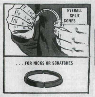
'Course, the cone gaps are equally spaced during installation so that the main rotor can seat properly. After the jesus nut is tightened no further maintenance is needed on the cones, even if they slip and touch during operation.
