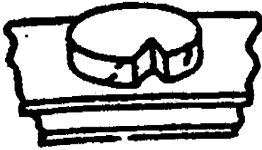
BURST CRACK DUE TO OVERHEATING UNACCEPTABLE
