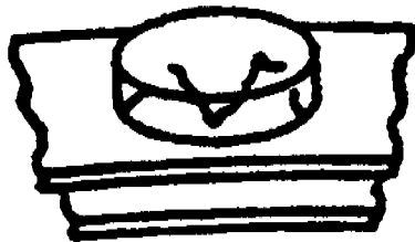
CRACKS DUE TO EXCESSIVE COLD WORKING ARE UNACCEPTABLE IF THERE ARE MORE THAN 3 NON INTERSECTING CRACKS
