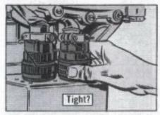
Press the press-to-test switch. Illumination means the light and electrical system are OK.
