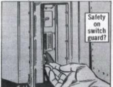
Check all electrical connectors and switches to make sure they're tight and undamaged.
