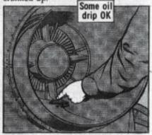
When is oil leakage excessive? When consumption is more than 2.4 pints per hour, according to Table 4-1 -item 28-in TM 55-2840-229-24
