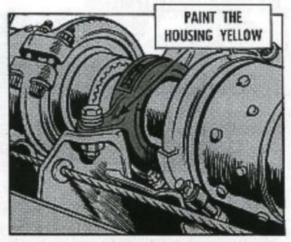
Your Huey PMD calls for a damage and security check on the tail rotor shafts, hangers, clamps and covers plus an inspection for grease leakage on all tail rotor shaft couplings . . . no sweat.
