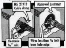
Following these rules should lengthen cable life by preventing excessive bend stresses and chafing. That's why they were included in Section XI of TM 11-530 (Dec 59), which is the Army's guide on "Installation Practices for Aircraft Electric and Electronic Wiring." See if you can pick up a copy.
