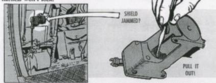
When this happens, use a gizmo, gadget, or whatchamacallit to reach behind the shield and pull it back out of the locking dog area. If the shield comes loose don't fret—just push it back into position.
