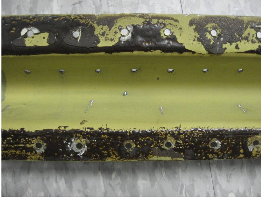
Figure 1 Drill damage to inside of Longeron (Longeron removed)
