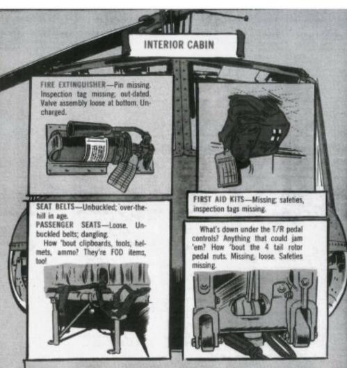
One last tip: Any bolt or nut you can hand turn is suspect. Just be sure that you doublecheck any that's not supposed to turn.
