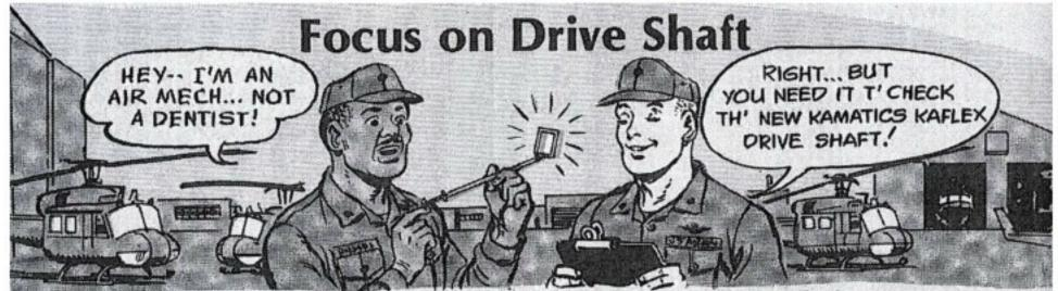
Use an inspection mirror to eyeball the flexible-plate main drive shaft during the PM Daily, Huey mechs. The added check is for birds with the new Kamatics Kaflex drive shaft. TSARCOM Msg DRSTS-MEA 101745Z Apr 81 (UH-1-81-05) has details.
