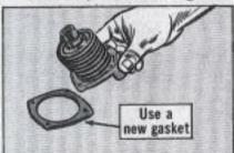
NSN 5330-00-107-5393. Remember that the filter is on the pressure side of the oil pump and the gasket has to hold.
