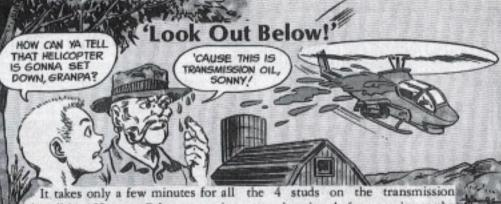
sion to squirt past a blown oil filter filter. gasket. And with a drop in oil pressure, the pilot has to set 'er down before the transmission seizes up.
