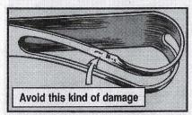
Using any kind of lever—like a screwdriver—could bend the bleed band. Then it won't be able to move in the narrow space available.
