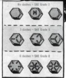
a medium torque. Six dash (Grade 8) capscrews are made out of carbon-alloy steel. They're the strongest kind you're likely to see in ground equipment and take the highest torque.
