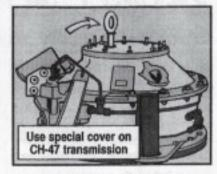
that comes with the transmission. It keeps moisture out and holds the planetary gears safely in place.
