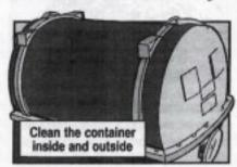
or by steam cleaning. That'll get rid of all dirt, sand and grease. Replace damaged or missing hardware with the items listed in TB 55-8100-200-24. Maintenance of Specialized Reusable Containers for Aircraft Equipment.
