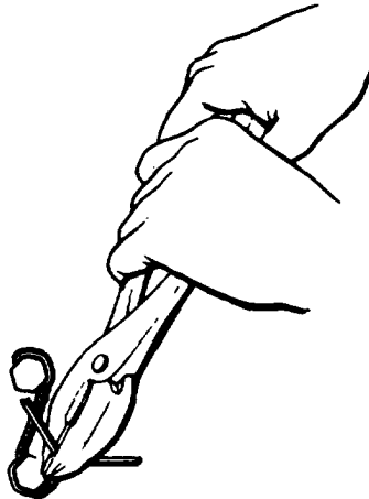
8. BENDING TWISTED WIRE
