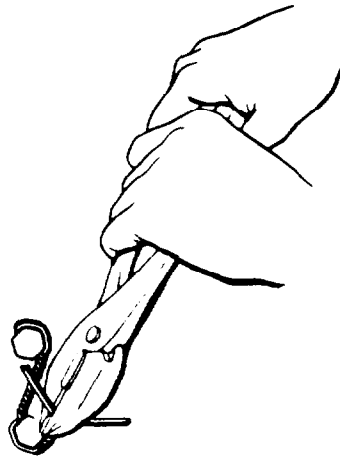
8. BENDING TWISTED WIRE
