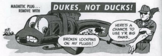
Removing the magnetic chip detector insert plug at the Huey (UH-1) 42" gear box is a hands-only job—not one for pliers!
