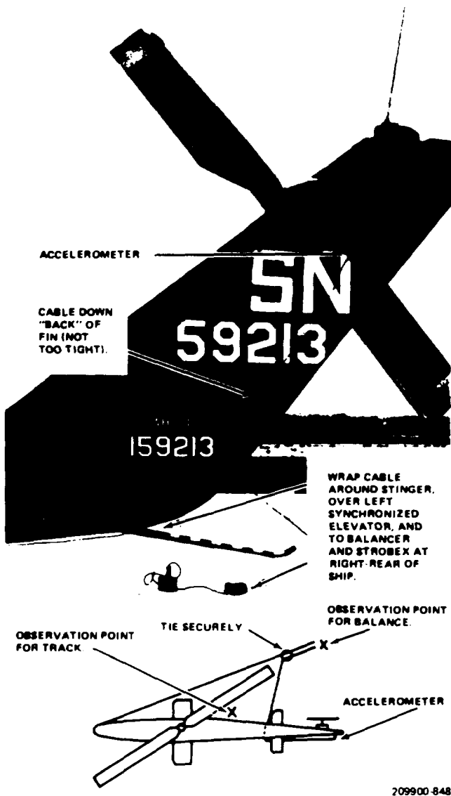
Figure 5-115. Accelerometer Cable Installation (Typical)
