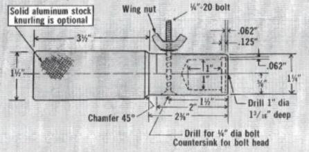
We made our puller from 1½-in aluminum round stock, about 6 inches long. It's real easy to make and will prevent glasses from being damaged from using other removal methods...saves on replacement costs.
