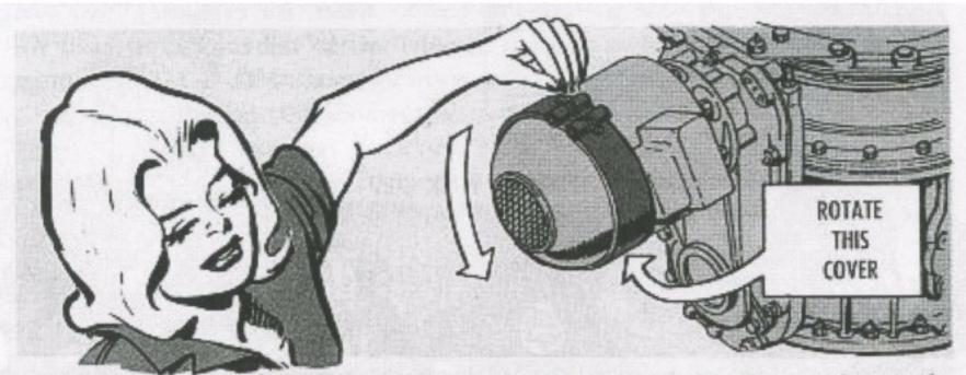
If brush cover, P/N 30010-1035, is bolted together with the opening at the top of the generator, slip the cover 180 degrees so that it's at the bottom. Then water won't leak into the generator and short out the works.
